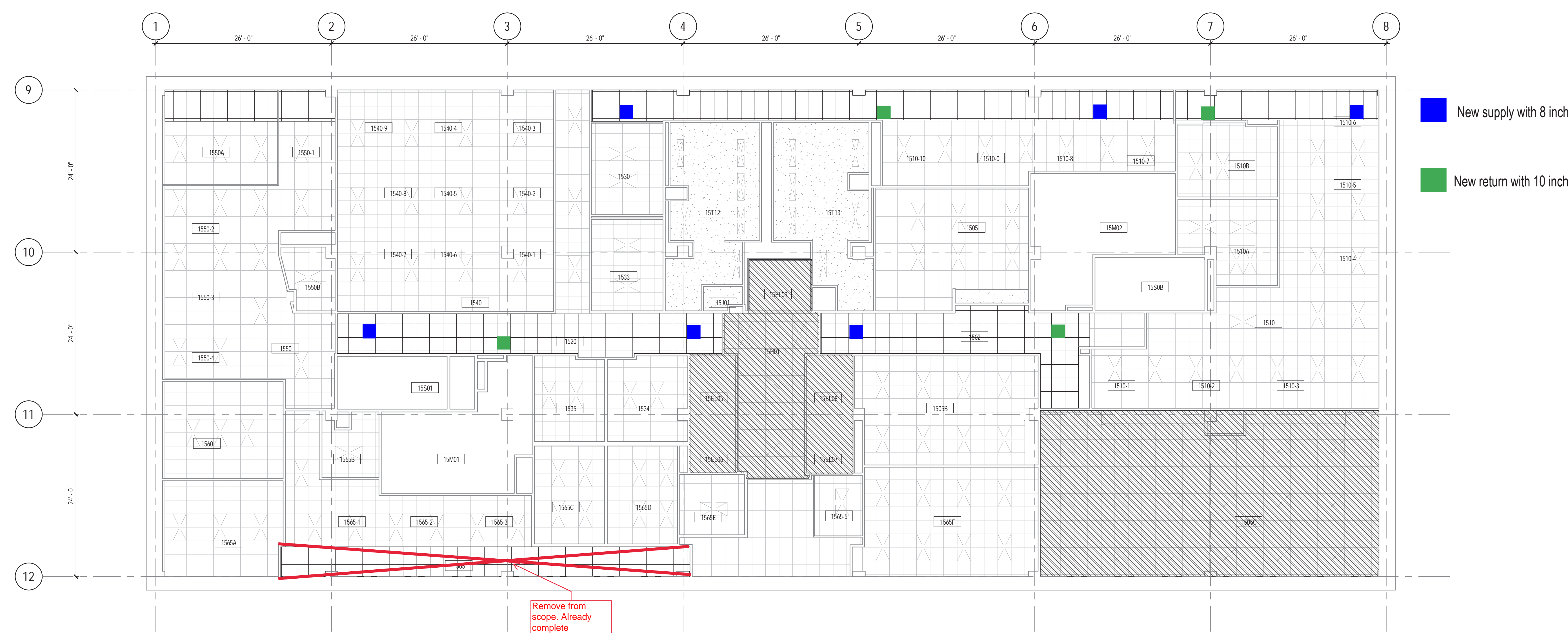
1 NEW REFLECTED CEILING PLAN - LEVEL 15 1/8" = 1'-0"
